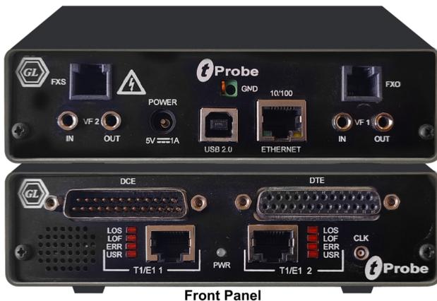
Figure: tProbe™ FXO FXS Simulator
